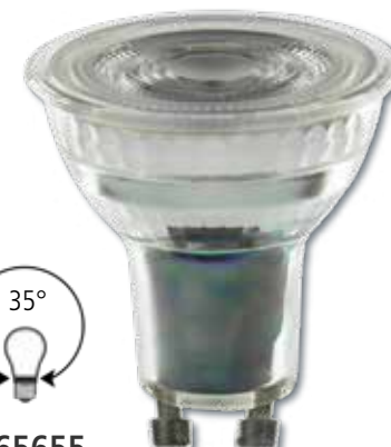
TR-65655 LED Reflector GU10 6,8 W / 510 lm / 2700 K
