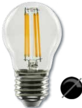
TR-65609 LED Golf Ball clear 4,5 W / 470 lm / 2700 K TUNGSRAM
