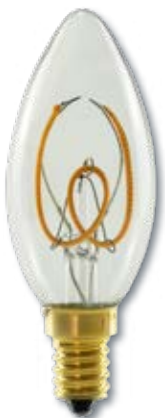
SG-50630 LED Soft Candle clear 3,2 W / 190 lm / 2200 K
